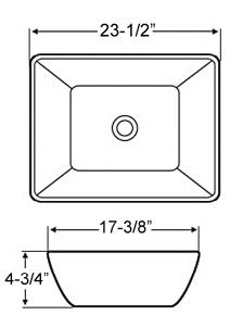
Dimensions of fixture are nominal and may vary within the range of tolerances established by AMSE Standard A112.19.2.2013 Dimensions and specifications subject to change without notice.
